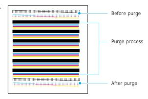
6. If the line is still broken, clean the print nozzles. See "Cleaning the Print Cartridge Nozzles" on page 6.5.
